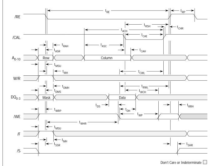
NOTES: 1. Data mask bit high (1) enables bit write; data mask bit low (0) inhibits bit write.
