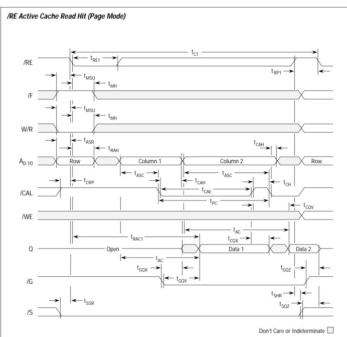
NOTES: 1. If column address 2 modifies only address pin A<sub>9</sub> or A<sub>10</sub>, then  $t_{AC}$  becomes  $t_{AC1}$  for data 2 and  $t_{CQX}$  becomes  $t_{CQX1}$  for data 1.
