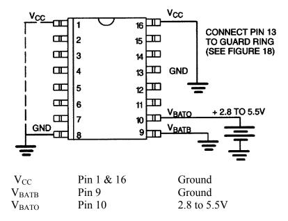
The  $V_{BATO}$  pin is normally connected to any standard 3 V lithium cell or other energy source. The Battery Operate mode also minimizes the power-consumption in applications where battery backup is not required and the  $V_{BATO}$  lead is directly connected to the system's 5V supply.
