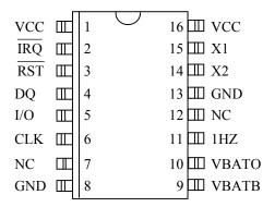
16-PIN DIP (300 MIL) 16-PIN SOIC (300 MIL) 16-PIN SSOP (208 MIL)
