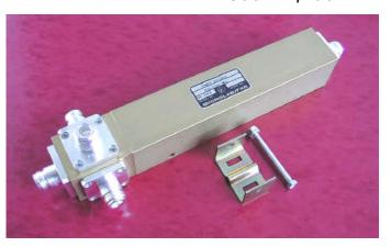
Microlab/FXR Model D4-24FN Four Way Power Splitter with N connectors, has been designed to evenly split high power cellular signals with minimal reflections or loss. All joints are sealed with O-rings to seal out moisture. The mechanical shape allows simple attachment to pole or wall using the bracket provided.
