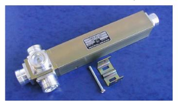
Microlab/FXR Model D4-24FD Four Way Power Splitter with 7-16 mm DIN connectors, has been designed to evenly split high power cellular signals with minimal reflections or loss. All joints are sealed with Orings to seal out moisture. The mechanical shape allows simple attachment to pole or wall using the bracket provided.
