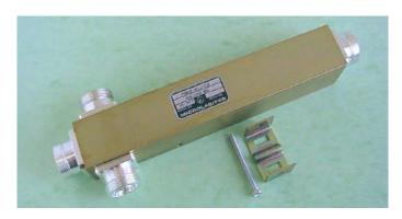
Microlab/FXR Model D3-24FD Three Way Power Splitter with 7-16 mm DIN connectors has been designed to evenly split high power cellular signals with minimal reflections, passive intermodulation or loss. All joints are sealed with Orings to seal out moisture. The mechanical shape allows simple attachment to pole or wall using the bracket provided.
