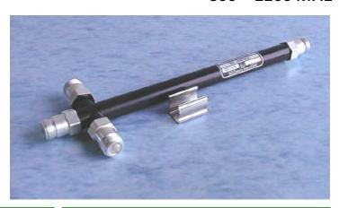
Microlab/FXR Model D3-14FN Three Way Power Splitter has been designed to evenly split high power, cellular signals with minimal reflections or loss. Its convenient, mechanical shape allows simple attachment to pole or wall using the accessory spring clip, and since the unit is weatherproofed it may be used for both indoor and outdoor applications. Designed with only a few solder joints and an air dielectric, the loss has been minimized and reliability enhanced.
