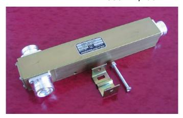
Microlab/FXR Model D2-24FD Two Way Power Splitter has been designed to evenly split high power cellular signals with minimal reflections or loss. All joints are sealed with O-rings to seal out moisture. The mechanical shape allows simple attachment to pole or wall using the supplied bracket accessory.
