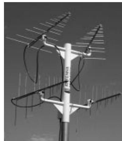
E. **DFA-350**, Antenna System offering a frequency range of 100 MHz to 5 GHz suitable for receiving both horizontal and vertical polarization. This antenna is also suited for generating sum and difference radiation pattern for direction finding.
