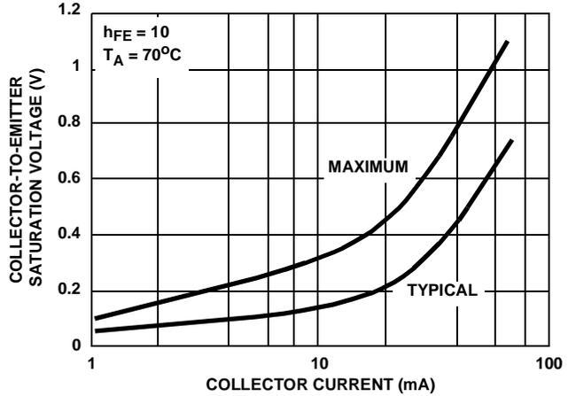
FIGURE 6. COLLECTOR-TO-EMITTER SATURATION VOLTAGE vs COLLECTOR CURRENT
