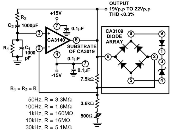
**FIGURE 22. WIEN BRIDGE OSCILLATOR CIRCUIT USING CA3140**
