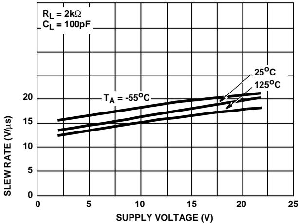
FIGURE 31. SLEW RATE vs SUPPLY VOLTAGE AND TEMPERATURE
