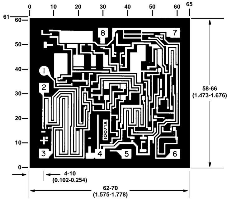
Dimensions in parenthesis are in millimeters and are derived from the basic inch dimensions as indicated. Grid graduations are in mils ( $10^{-3}$  inch).
