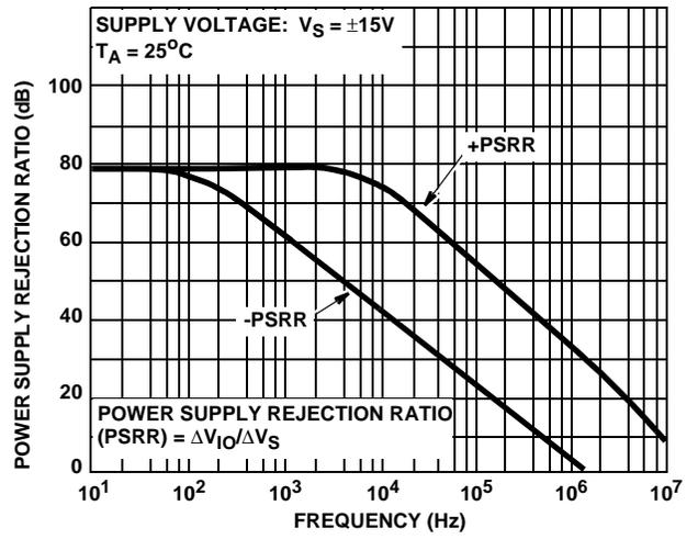
FIGURE 36. POWER SUPPLY REJECTION RATIO vs FREQUENCY
