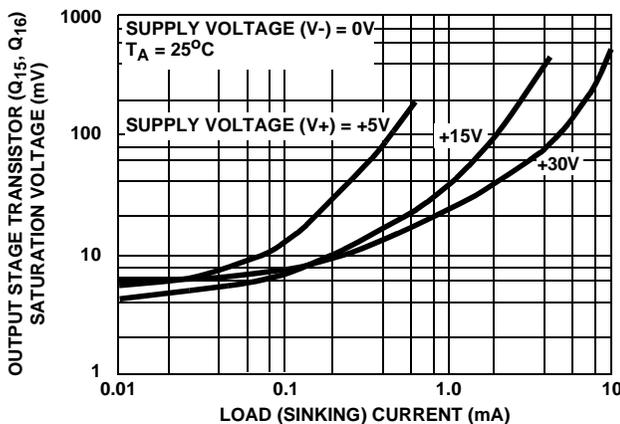
**FIGURE 2. VOLTAGE ACROSS OUTPUT TRANSISTORS (Q<sub>15</sub> AND Q<sub>16</sub>) vs LOAD CURRENT**
