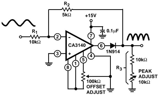
$$\text{GAIN} = \frac{R_2}{R_1} = X = \frac{R_3}{R_1 R_2 + R_3}$$
