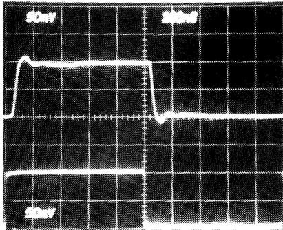
Top Trace: Output;  $50\text{mV}/\text{Div.}$ ,  $200\text{ns}/\text{Div.}$
