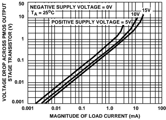
FIGURE 22. VOLTAGE ACROSS PMOS OUTPUT TRANSISTOR (Q<sub>8</sub>) vs LOAD CURRENT
