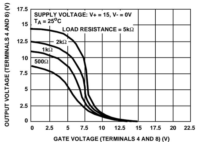
FIGURE 2. VOLTAGE TRANSFER CHARACTERISTICS OF CMOS OUTPUT STAGE
