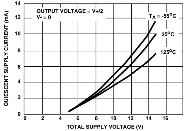
FIGURE 21. QUIESCENT SUPPLY CURRENT vs SUPPLY VOLTAGE
