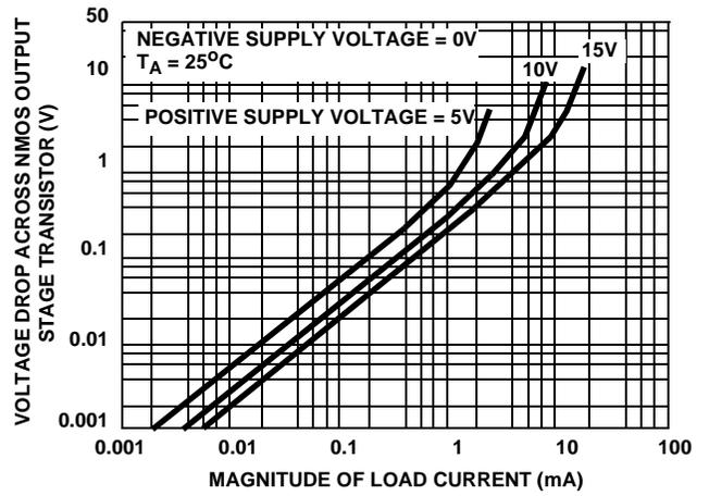
FIGURE 23. VOLTAGE ACROSS NMOS OUTPUT TRANSISTOR (Q<sub>12</sub>) vs LOAD CURRENT
