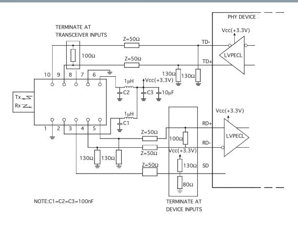
The split-loaded terminations for ECL signals need to be located at the input of devices receiving those ECL signals. The power supply filtering is required for good EMI performance. Use short tracks from the inductor L1/L2 to the module Rx Vcc. A GND plane under the module is required for good EMI and sensitivity performance.
