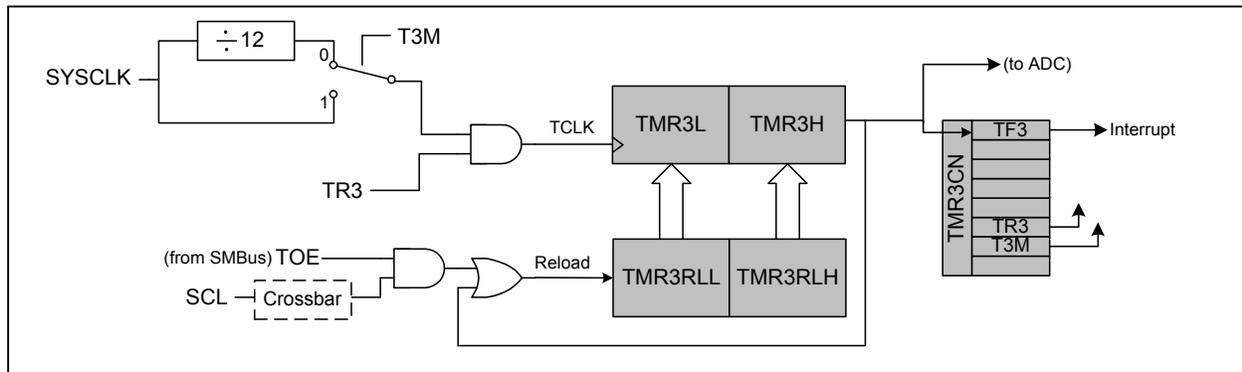
**Figure 19.20. TMR3CN: Timer 3 Control Register**
