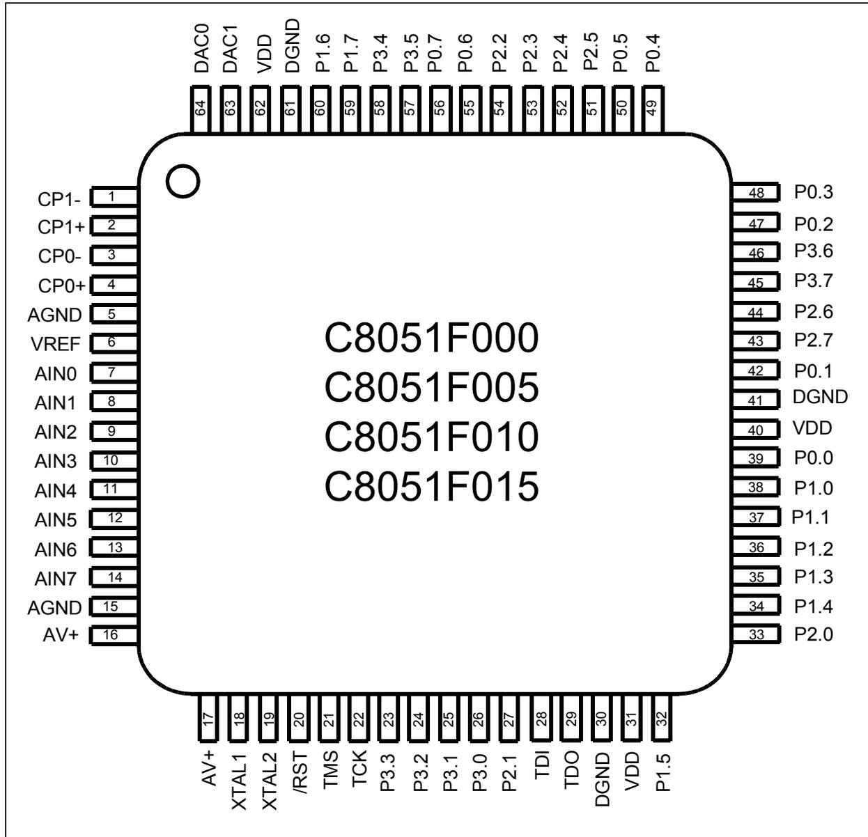
**Figure 4.2. TQFP-64 Package Drawing**
