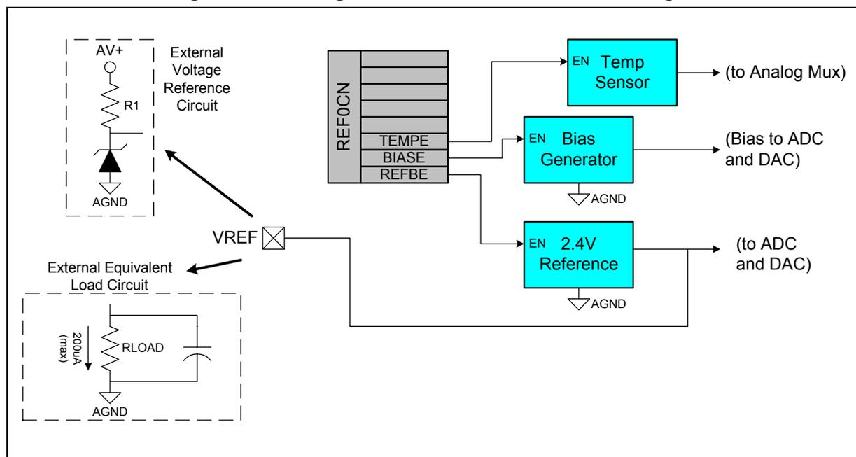
**Figure 9.2. REF0CN: Reference Control Register**
