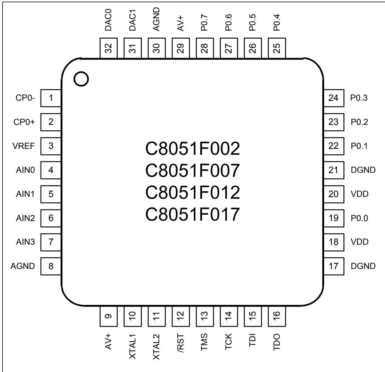
**Figure 4.6. LQFP-32 Package Drawing**
