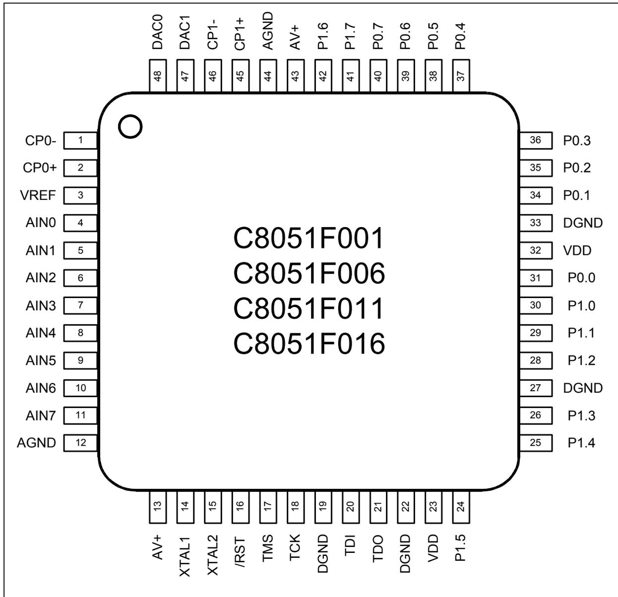
**Figure 4.4. TQFP-48 Package Drawing**
