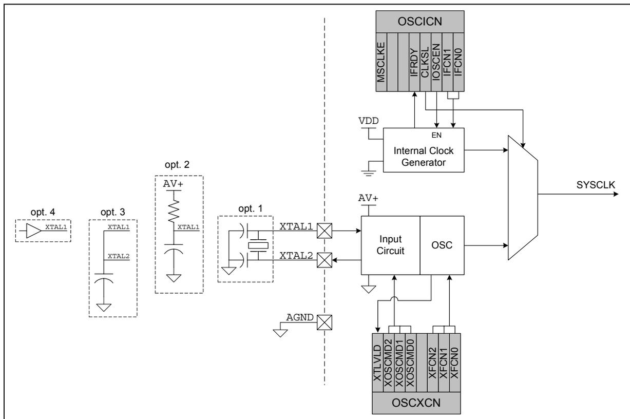
Figure 14.2. OSCICN: Internal Oscillator Control Register
