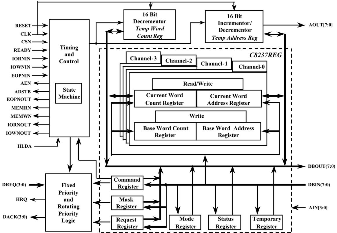
Figure 1: C8237 Programmable DMA Controller Block Diagram
