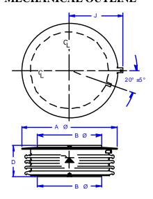
$A\Phi = 2.30 \text{ in } (58.0 \text{ mm})$   $B\Phi = 1.35 \text{ in } (34.3 \text{ mm})$ D = 1.04 in (26.4 mm)
