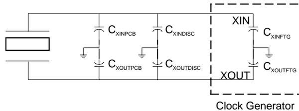
As an example, and using this formula for this datasheet's device, a design that has no discrete loading capacitors ( $C_{DISC}$ ) and each of the crystal to device PCB traces has a capacitance ( $C_{PCB}$ ) to ground of 4pF (typical value) would calculate as:
