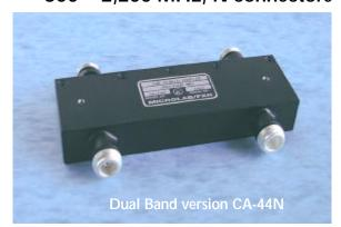
The CA-34N, -44N and -54N Hybrid Couplers have been designed to meet the special needs of the wireless market. They are most commonly used to combine two wireless carriers to a single antenna feed or distribution cable. This requires the termination of one output port in  $50\Omega$  and results in a 3 dB loss in each signal. In situations where two similar feeds are required, for say an in-building application, both outputs may be used, eliminating the need for a termination and the 3 dB loss.
