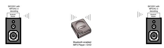
The BIC2201 incorporates an integrated dual ARC3 RISC processor architecture with embedded DSP to support the Bluetooth<sup>TM</sup> Protocol stack for the wireless link, as well as a variety of Multimedia Compression Techniques.
