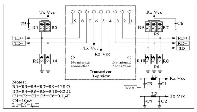
The split-loaded terminations for ECL signals need to be located at the input of devices receiving those ECL signals. The power supply filtering is required for good EMI performance. Use short tracks from the inductor L1/L2 to the module Rx Vcc. A GND plane under the module is required for good EMI and sensitivity performance.
