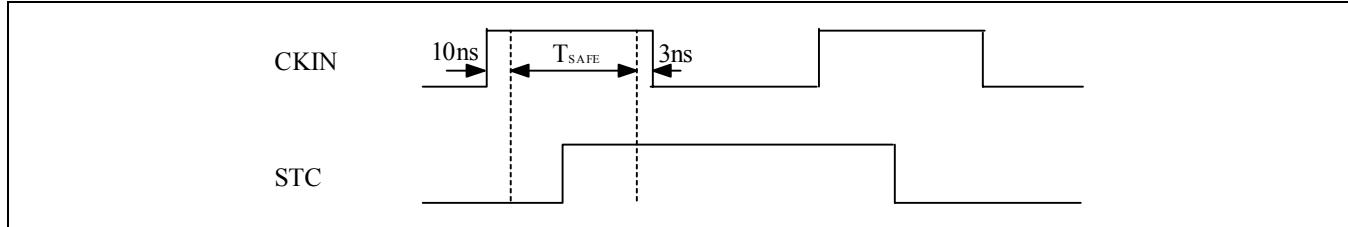
The A/D Converter operates data conversion when STC (Start Conversion) signal is just "HIGH". Otherwise, output data (DO[11:0]) keep the current states. The STC signal should be changed during " $T_{SAFE}$ " with the "HIGH" level of the clock to operation as shown in the main waveform.
