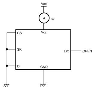
Fig.8 Standby current circuit
