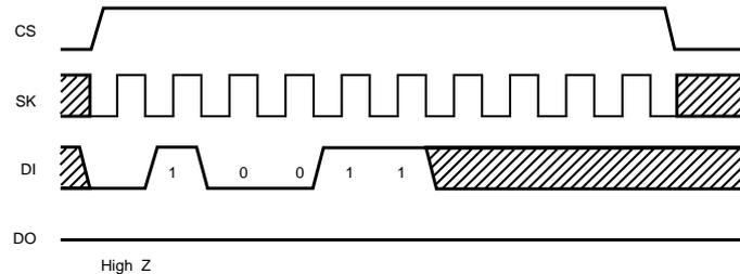
Fig.11 Write enable cycle timing
