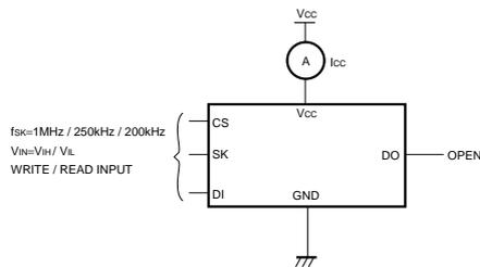
Fig.7 Supply current circuit
