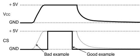
(Bad example) Here, the CS pin is pulled up to V<sub>cc</sub>. In this case, CS is HIGH (active state). Please be aware that the EEPROM may perform erroneous operations or write erroneous data because of noise or other factors. Please be aware that this can occur even if the CS input is HIGH-Z.
