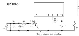
For acutual usage, Please kindly evaluate and confirm our part mounted in your product, Especially, Please make sure to confirm the load current does not exceed Max. rated current by using the current probe.
