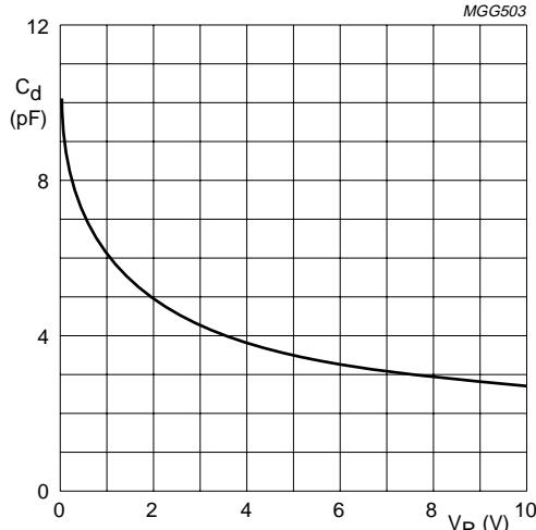
$f = 1 \text{ MHz}; T_j = 25^\circ\text{C}.$
