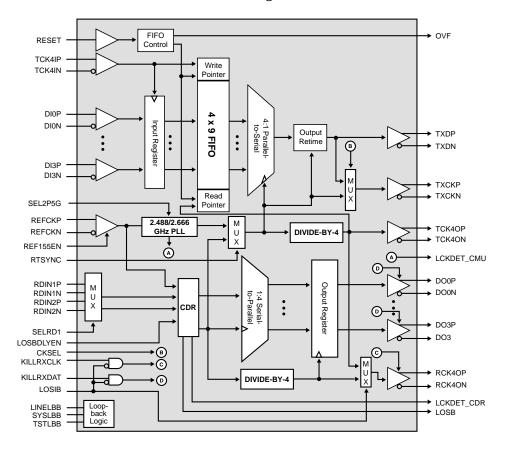
The **BCM8220** FEC-capable (Forward Error Correction), SONET/SDH transceiver is a fully integrated, SONET OC-48 (2.488/2.667 Gbps) interface serialization/deserialization device with an integrated clock multiplication unit (CMU) and integrated clock and data recovery (CDR) circuit. Output frequency is selectable at 2.488 Gbps or 2.667 Gbps, allowing use of the FEC capability.
