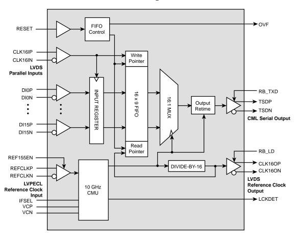
The **BCM8110** is a fully integrated SONET/SDH transmitter operating at data rate of 9.953 Gbps with serializer, Clock Multiplication Unit (CMU), and Loss-of-Signal (LOS) detection circuitry. The low-jitter LVDS interface and the onboard low-jitter PLL meets Optical Internetworking Forum (OIF), IEEE 802.3ae, Telcordia, ANSI, and ITU-T jitter standards.
