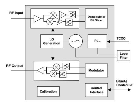
The **BCM2002** Bluetooth<sup>™</sup> transceiver is an integrated radio transceiver that is optimized for use in 2.4-GHz Bluetooth wireless systems. The transceiver is Bluetooth 1.1 compliant and is designed to be compatible with Bluetooth-enabled CDMA chipsets.
