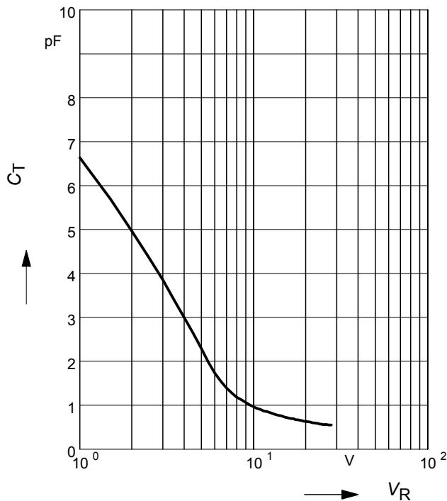
**Normalized diode capacitance**
