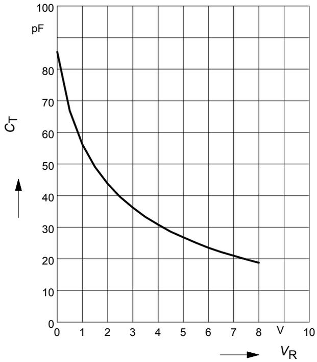
**Capacitance ratio  $C_{Tref}/C_T = f(V_R)$**
