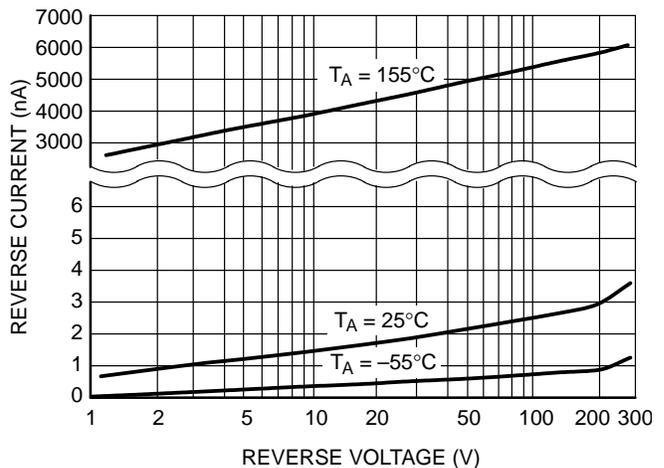
Figure 3. Reverse Leakage
