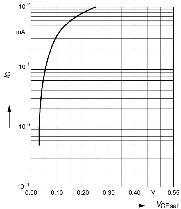
**Input off voltage**  $V_{i(off)} = f(I_C)$
