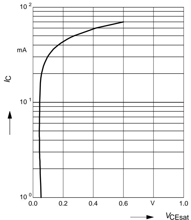
**Input on Voltage**  $V_{i(on)} = f(I_C)$
