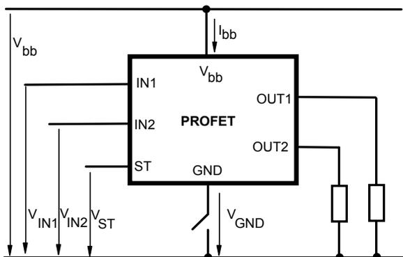
Any kind of load. In case of IN=high is  $V_{OUT} \approx V_{IN} - V_{IN(T+)}$ .
