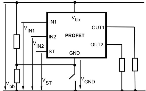
Any kind of load. If  $V_{GND} > V_{IN} - V_{IN(T+)}$  device stays off
