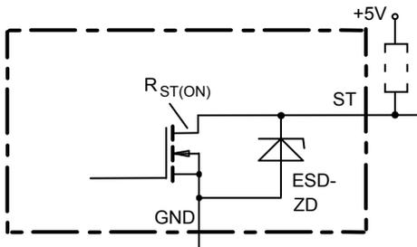
ESD-Zener diode: 6.1 V typ., max 5.0 mA;  $R_{ST(ON)} < 380 \Omega$  at 1.6 mA, ESD zener diodes are not to be used as voltage clamp at DC conditions. Operation in this mode may result in a drift of the zener voltage (increase of up to 1 V).
