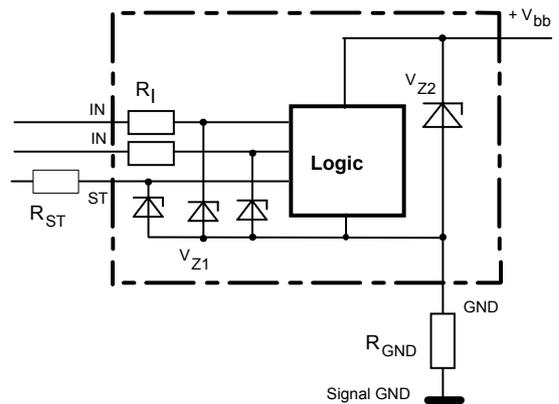
$V_{Z1} = 6.1 \text{ V typ.}$ ,  $V_{Z2} = 47 \text{ V typ.}$ ,  $R_I = 3.5 \text{ k}\Omega \text{ typ.}$ ,  $R_{GND} = 150 \Omega$
