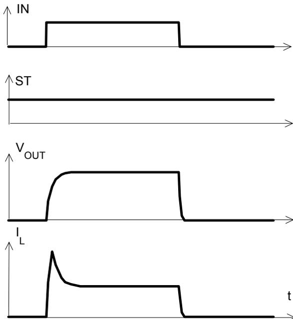
The initial peak current should be limited by the lamp and not by the initial short circuit current  $I_{L(SCp)} = 7.5 \text{ A typ.}$  of the device.
