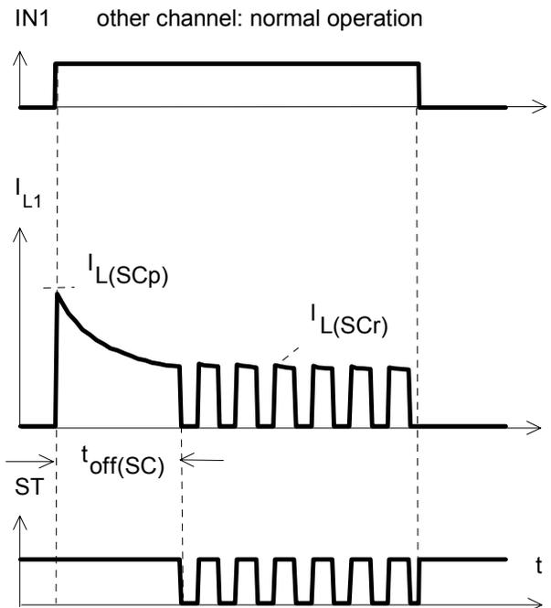
Heating up of the chip may require several milliseconds, depending on external conditions ( $t_{off(SC)}$  vs.  $T_{j,start}$  see page 11)
