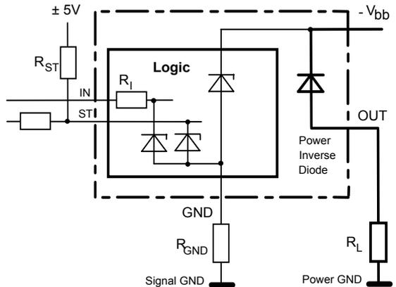
$R_{GND} = 150 \Omega$ ,  $R_I = 3.5 \text{ k}\Omega \text{ typ.}$
