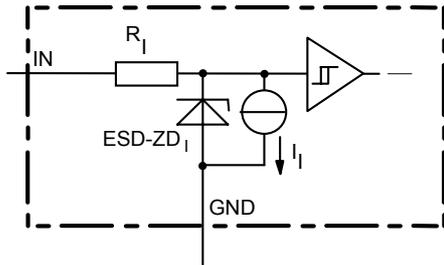
ESD zener diodes are not to be used as voltage clamp at DC conditions. Operation in this mode may result in a drift of the zener voltage (increase of up to 1 V).
