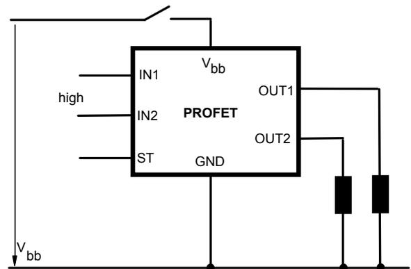
For an inductive load current up to the limit defined by  $E_{AS}$  (max. ratings see page 3 and diagram on page 10) each switch is protected against loss of  $V_{bb}$ .
