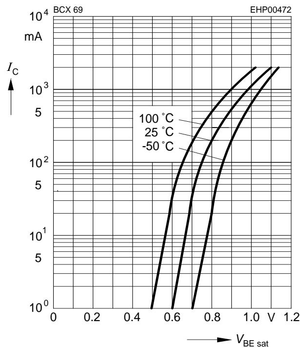
**Collector current**  $I_C = f(V_{BE})$
