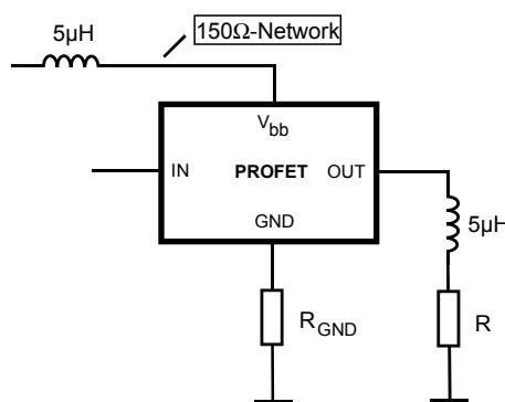
For defined decoupling and high reproducibility a defined choke (5µH at 1 MHz) is inserted between supply and  $V_{bb}$ -pin.
