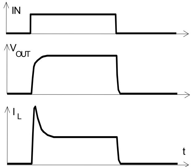
**Figure 2a:** Switching a resistive load,
