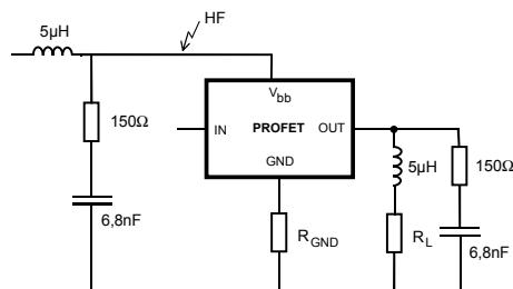
For defined decoupling and high reproducibility the same choke and the same 150Ω -matching network as for the emission measurement is used.
