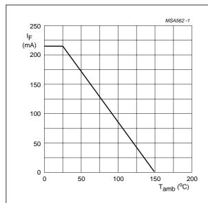
Device mounted on an FR4 printed-circuit board.
