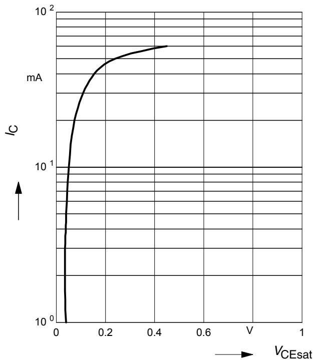
**Input off voltage**  $V_{i(off)} = f(I_C)$
