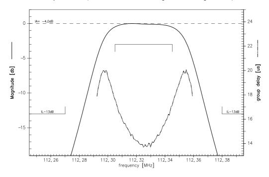
Transfer function wide band (normalized, measurement single-ended / single-ended)
