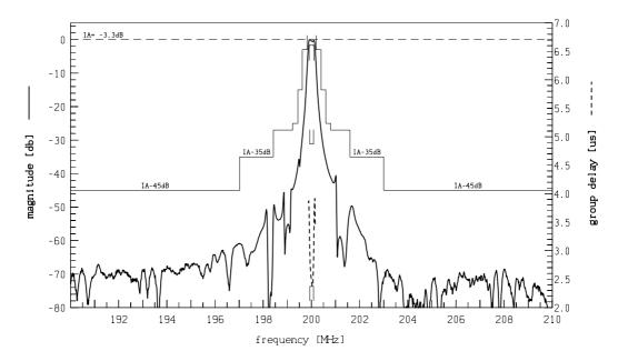
**Transfer function** - passband (measured in test matching network to 50  $\Omega$ ):
