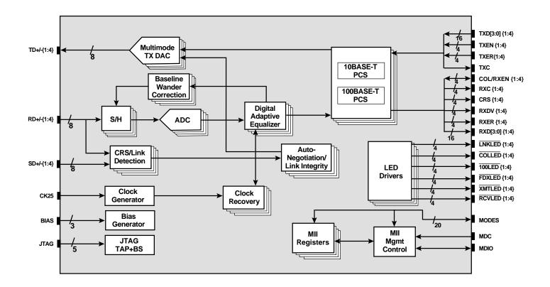
The **BCM5208** is a monolithic CMOS integrated circuit containing four transceivers that each perform all the physical layer interface functions for 10BASE-T Ethernet on CAT 3, 4, 5 unshielded twisted pair (UTP) cable, 100BASE-TX Ethernet on CAT5 UTP cable, and 100BASE-FX Ethernet on 62.5/125- $\mu$ m multimode fiber optic cable.
