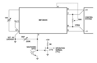
The above diagram shows the remote sense feature which reduces Vo errors due to the resistance of the conductors feeding the load. This diagram also shows the connections for non-synchronized operation (TIMING 1 and 2) as well as output voltage trim, remote shutdown, fault monitoring, and input voltage turn on point adjustment.
