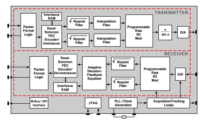
The **BCM6315** is a single-chip V-thernet<sup>TM</sup> transceiver design based on many years experience of QAM technology and LAN products. It is designed for low-cost, long-reach Ethernet applications employing telephone-grade wiring. The **BCM6315** offers switch, DSLAM and CPE vendors an unmatched capability for the provision of high-speed data transmission services such as Internet access and LAN extensions in MDU, MTU, hospitality and campus environments.
