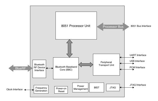
The BCM2039 architecture includes an enhanced 8051 processor core, on-chip boot ROM and SRAM, an intelligent software-hardware integrated baseband core, and standard input/output peripheral interfaces that include USB, UART, and PCM Audio Codec Serial Interface. The glueless connection to the BCM2001 Bluetooth Transceiver provides a complete, highly integrated Bluetooth solution.
