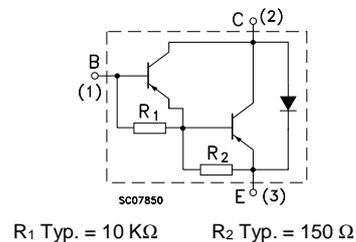
R<sub>1</sub> Typ. = 10 K $\Omega$       R<sub>2</sub> Typ. = 150  $\Omega$
