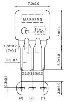
(1) : Input (2) : Ground (3) : Output (in mm)
