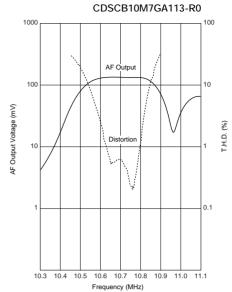
$\begin{array}{ll} \text{Input} &= 100 \text{ dB}\mu\\ \text{fdev.} &= \pm 75 \text{kHz}\\ \text{fmod.} &= 1 \text{kHz}\\ \text{Vcc} &= 1.2 \text{V} \end{array}$
