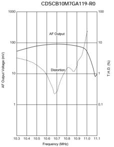
$\begin{array}{l} \text{Input} = 100 \text{ dB}\mu\\ \text{fdev.} = \pm 60 \text{kHz}\\ \text{fmod.} = 1 \text{kHz}\\ \text{Vcc} = 3.0 \text{V} \end{array}$
