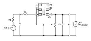
$$\begin{split} Rg &= 50\Omega \quad R1 = 280\Omega \pm 5\% \quad R2 = 330\Omega \pm 5\% \\ C2 &= 10 \pm 2 \text{ pF (Including stray capacitance and Input capacitance of RF Volt Meter)} \\ E1: S.S.G. Output Voltage ... \end{split}$$
