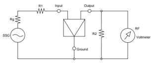
Rg+R1 =R2 : Input/Output Impedance
