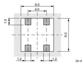
The material of P.C.B. is the epoxy resin of glass fabric base (t=0.8mm)
