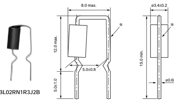
\*There is excess bond stick on the wire. (in mm)
