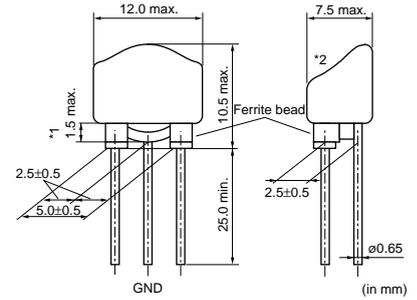
\*1 Coating extending on leads does not exceed the tangent line. Exposed electrode, if any, is covered by solder, etc.
