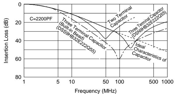
A three terminal capacitor has a higher self resonance frequency than a general two terminal type and exhibits effective noise suppression at high frequency.
