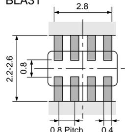
• If there are high amounts of self-heating on pattern, the contact points of PCB and part may become damaged.
