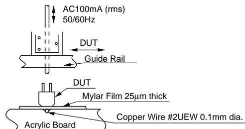
Fig. 2 Test Fixture for Output Voltage Measurement
