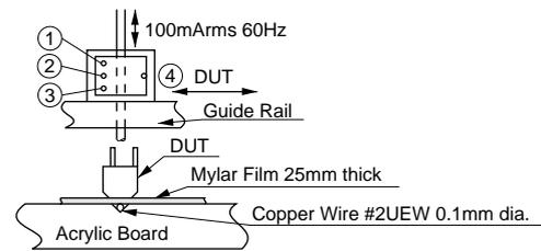
Fig. 2 Test Fixture for Output Voltage Measurement
