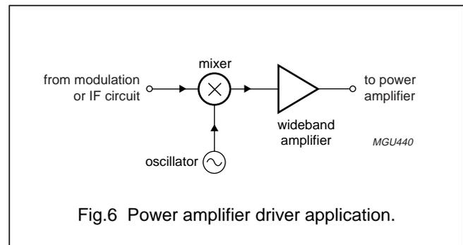
Fig.6 Power amplifier driver application.
