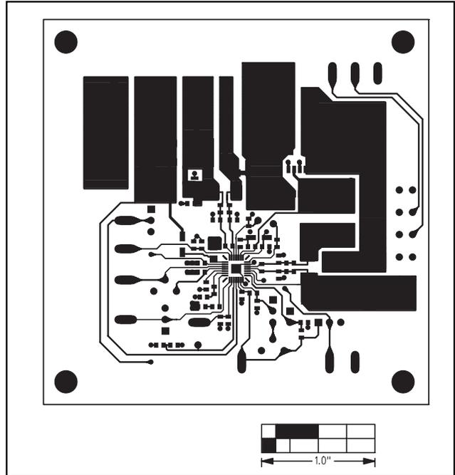
Figure 3. MAX1908 EV Kit PC Board Layout—Component Side
