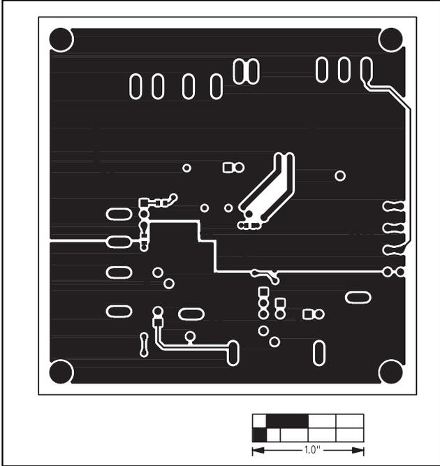
Figure 6. MAX1908 EV Kit PC Board Layout—Solder Side
