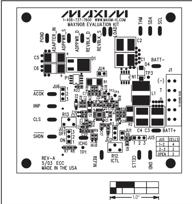
Figure 2. MAX1908 EV Kit Component Placement Guide—Component Side
