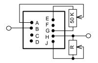
FULL SCALE ADJUST pin must be shorted to Output pin If trim pot is not used
